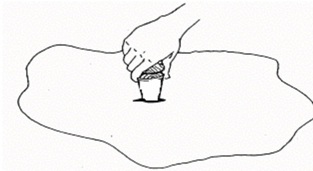
Installation of Wood Plug
